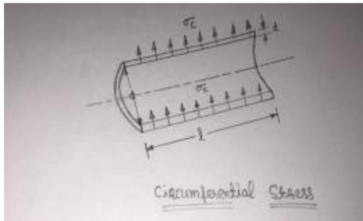
Let the hoop stresses develop due to the internal fluid pressure. The intensity of internal pressure is denoted by  $P$ . Due to the internal pressure, the shell may split up into two troughs along  $XX$  axis.
