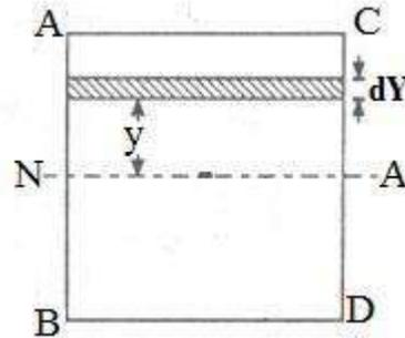
Let us assume one strip of thickness  $dy$  and area  $dA$  at a distance  $y$  from the neutral axis as displayed in above figure. Let us determine the force acting on the layer due to bending stress and we will have following equation
