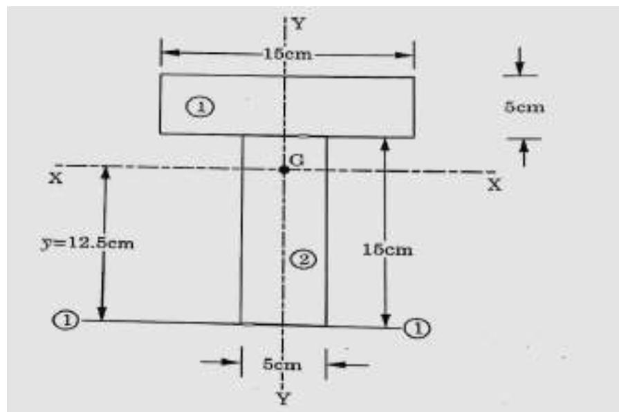
**Solution.** Let us split this T-section into two components- Component (1) and component (2).
