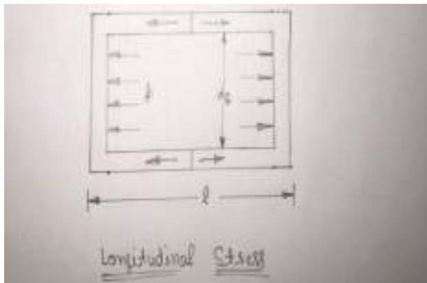
Bursting force =  $P \times \text{Area on which } P \text{ acts} = P \times (\pi d^2)$
