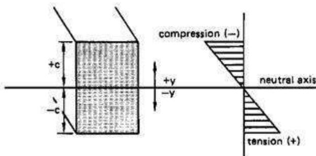
Figure Bending Stress Distribution in a Beam
