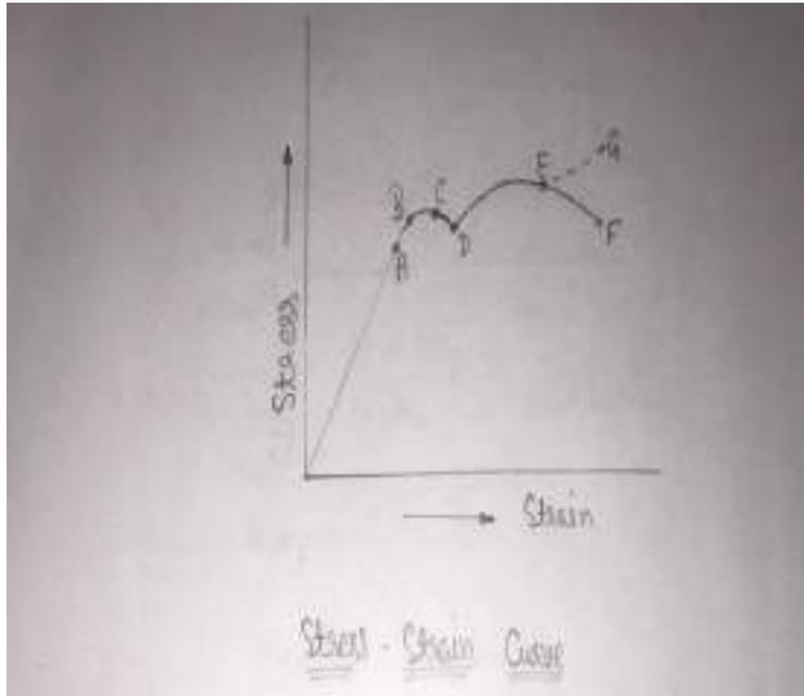
Figure shows that in stress-strain diagram for ductile materials, the curve starts from the origin, showing that there are no initial stresses or strain in the test specimen. The ductile specimen passes through the following stages during loading:-
