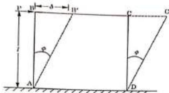
Fig. 2.3 : Strain Energy Stored Due to Shear Stress
