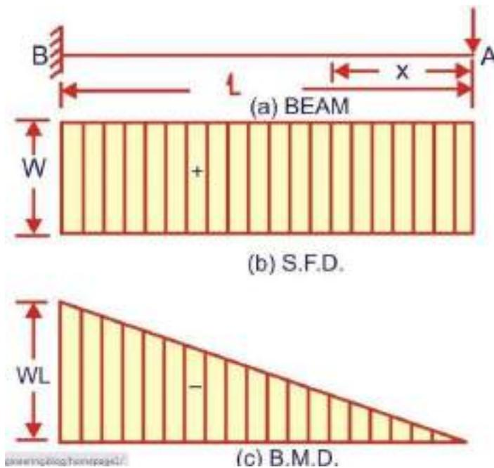
At section x from the end A,  $F_x = - Wl$  and is constant for any position of the section. The S.F.D. will, therefore, be rectangle of height W. Bending moment at a section x from end A is given by:
