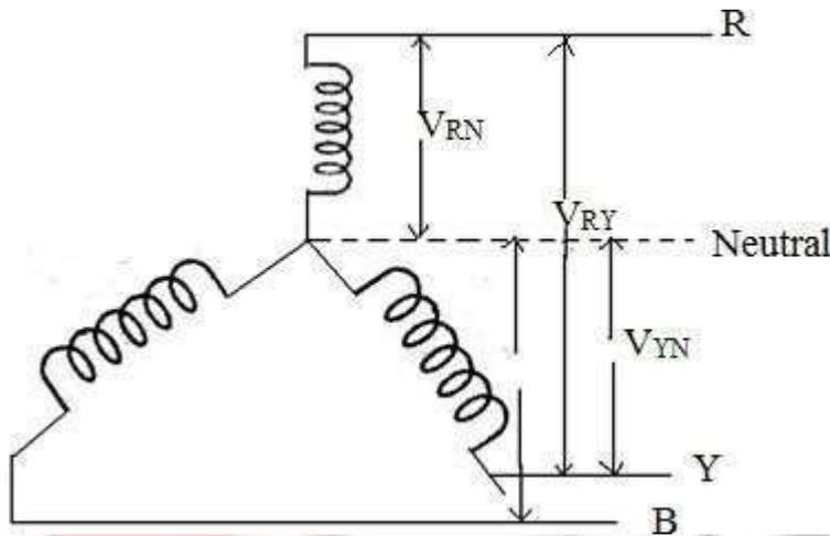
If three similar ends connected at one point, then it is known as star connected system.
