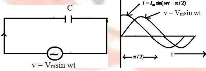
Let a capacitance of 'C' farad is connected across the A.C. supply of applied voltage
