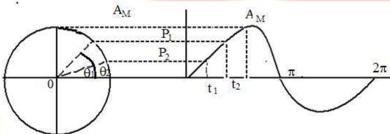
An alternating current or voltage, (quantity) in a vector quantity which has magnitude as well as direction. Let the alternating value of current be represented by the equation  $e = E_m \sin \omega t$ . The projection of  $E_m$  on Y-axis at any instant gives the instantaneous value of alternating current. Since the instantaneous values are continuously changing, so they are represented by a rotating vector or phasor. A phasor is a vector rotating at a constant angular velocity
