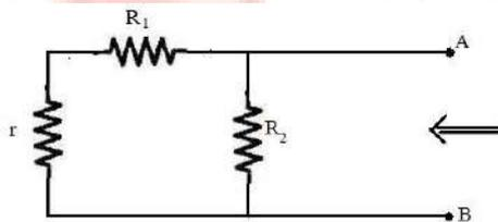
$$R_i = (R_1 + r) \parallel R_2 =$$
