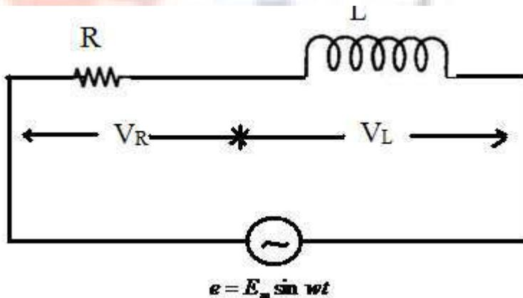
The resistance of  $R$ -ohm and inductance of  $L$ -henry are connected in series across the A.C. supply of applied voltage
