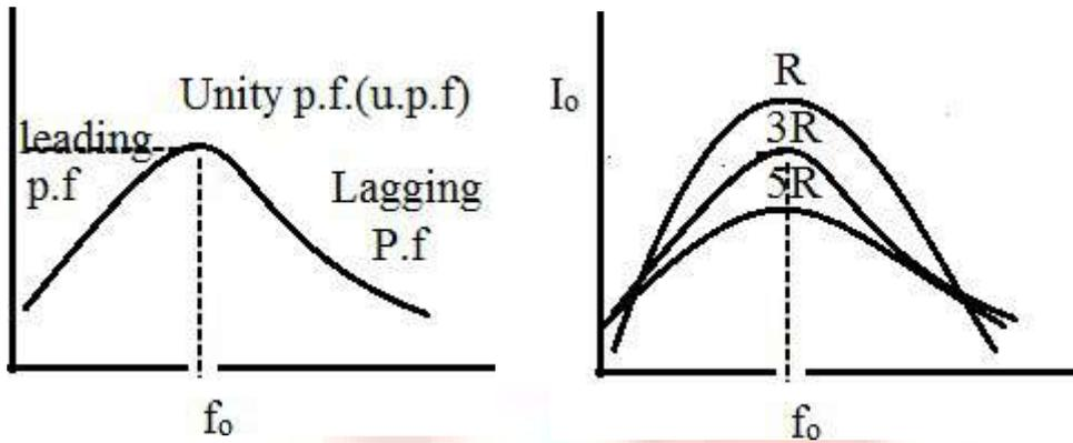
At low frequency the  $X_c$  is greater and the circuit behaves leading and at high frequency the  $X_L$  becomes high and the circuit behaves lagging circuit.
