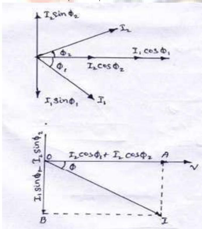
The resultant current “I” is the vector sum of the branch currents  $I_1$  &  $I_2$  can be found by using parallelogram law of vectors or resolving  $I_2$  into their X
