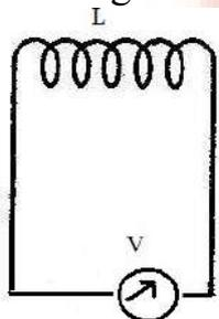
If current through the coil is changed then the flux linked with its own turn will also change which will produce an emf is called self-induced emf.
