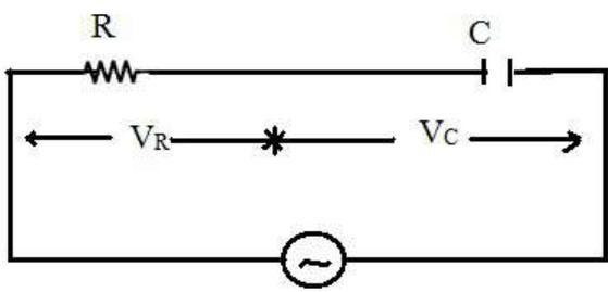
$$\begin{aligned} V &= V_R + (-jV_C) \\ &= IR + (-jIX_C) \\ &= I(R - jX_C) \\ V &= IZ \end{aligned}$$
