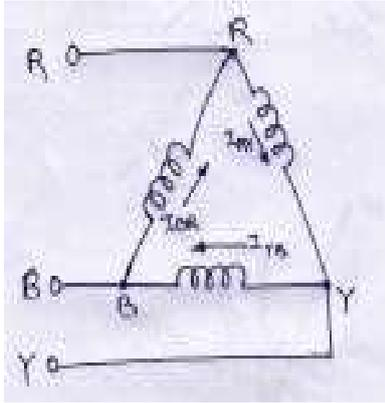
If the dissimilar ends of the closed mesh then it is called a Delta Connected system
