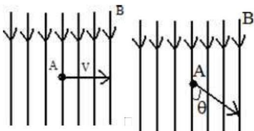
In this case the field is stationary and the conductors are rotating in an uniform magnetic field at flux density 'B' Wb/m<sup>2</sup> and the conductor is lying perpendicular to the magnetic field. Let 'l' is the length of the conductor and it moves a distance of 'dx' in time 'dt' second.
