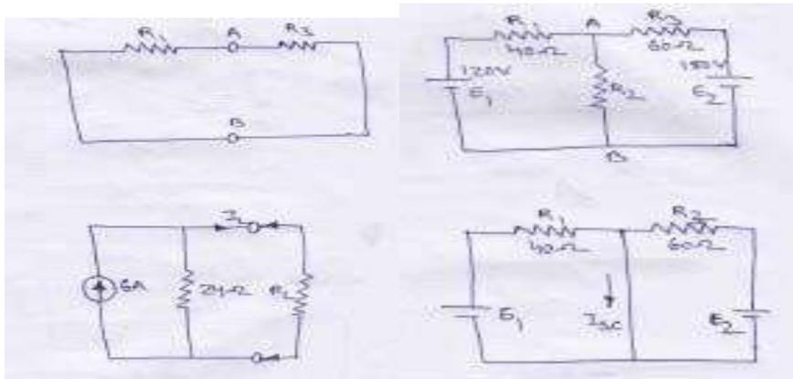
Step 01-remove the load resistance by making short circuit. now terminal AB short circuited.
