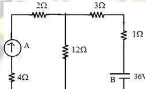
$$I = \frac{36}{8} = 4.5 \text{ Amp}, I = \frac{4.5 \times 12}{6 + 2} = 3 \text{ Amp} \text{ Transfer resistance} = \frac{V}{I} = \frac{36}{3} = 12 \Omega.$$
