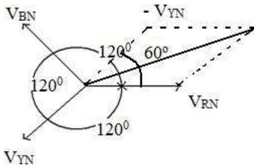
$$\begin{aligned} \text{Line Voltage } V_{RY} &= V_{RN} - V_{YN} \\ V_L &= \sqrt{V_{ph}^2 + V_{ph}^2 - 2V_{ph}V_{ph}\cos 60^\circ} \\ &= \sqrt{2V_{ph}^2 - 2V_{ph}^2 \times \frac{1}{2}} \\ &= \sqrt{3V_{ph}^2} = \sqrt{3}V_{ph} \\ V_L &= \sqrt{3}V_{ph} \end{aligned}$$
