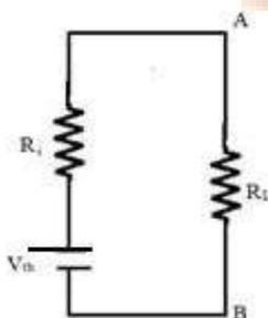
Connect internal resistances and Thevenin's voltage in series with load resistance  $R_L$ .
