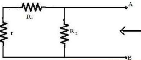
$$R_i = (R_1 + r) \parallel R_2$$
