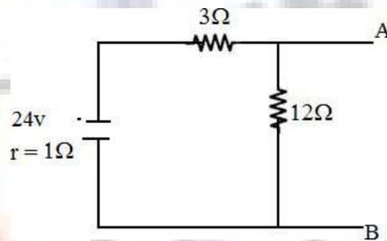
$V_{oc}$  is the voltage across  $12 \Omega$  resistor
