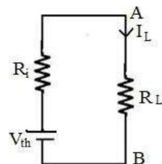
$$= \frac{V^2 R_L}{(R_i + R_L)^2}$$
