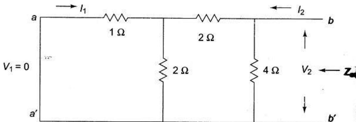
$$V_{22} = \left. \frac{I_2}{V_2} \right| V_1 = 0$$
